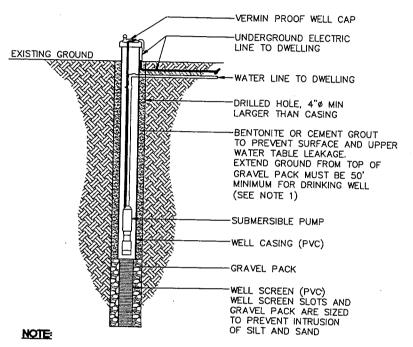
1. WELL DRILLER SHALL CONFIRM DEPTH OF WELL PRIOR TO INSTALLATION.
