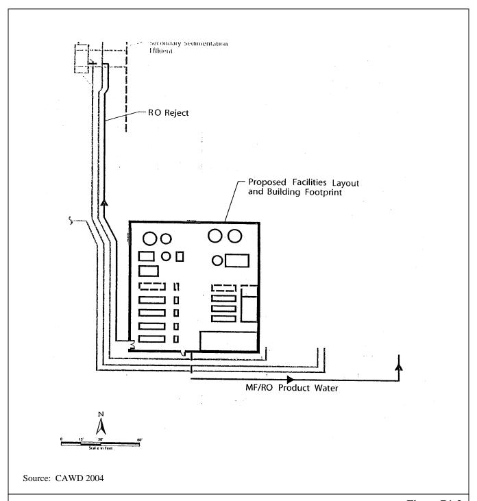
Figure P1-3 Recycled Water Project, Phase II Salinity Management Project Improvements at CAWD Plant
