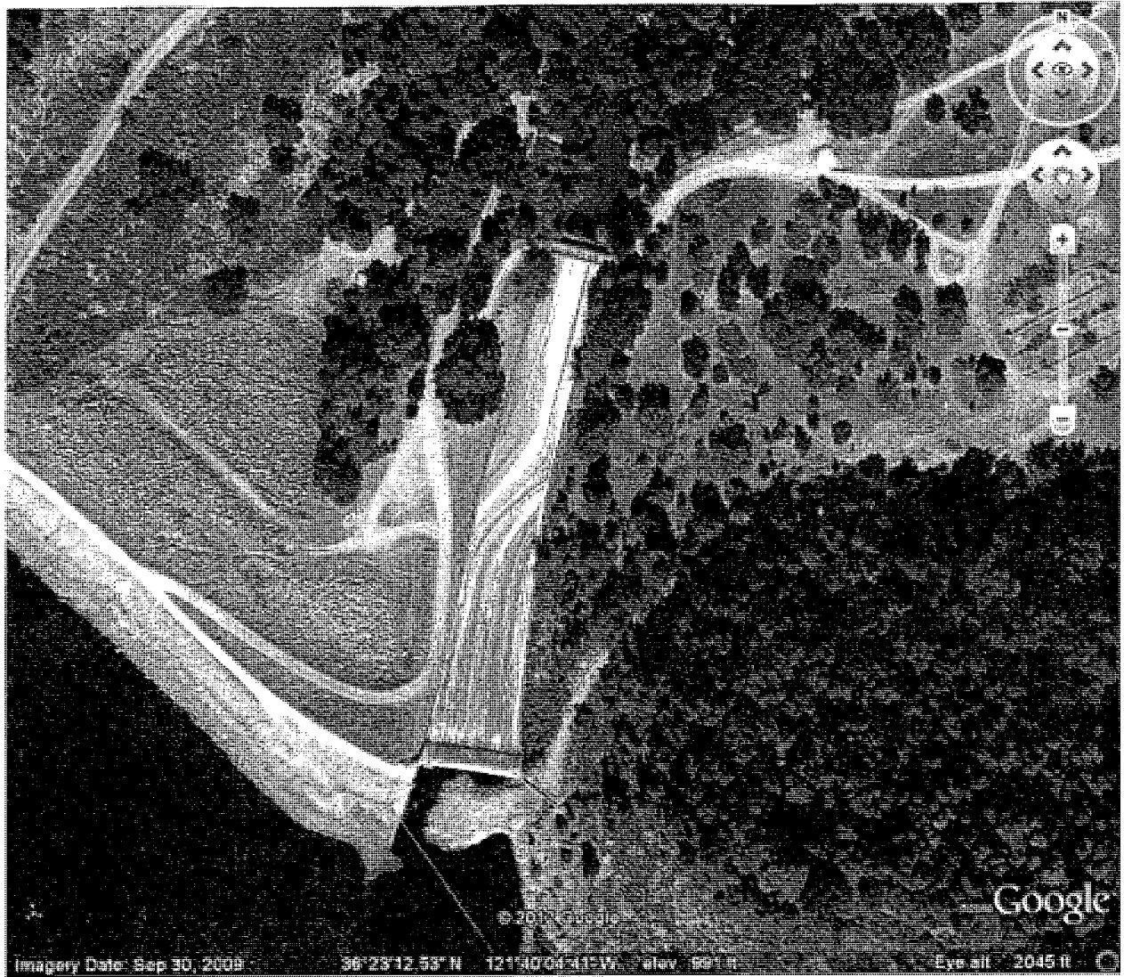
Satellite photo taken during low-water period (9-30-2009). Note inaccessible (dry) spillway preventing downstream passage. Similar conditions were noted during November 23, 2012 site visit.
